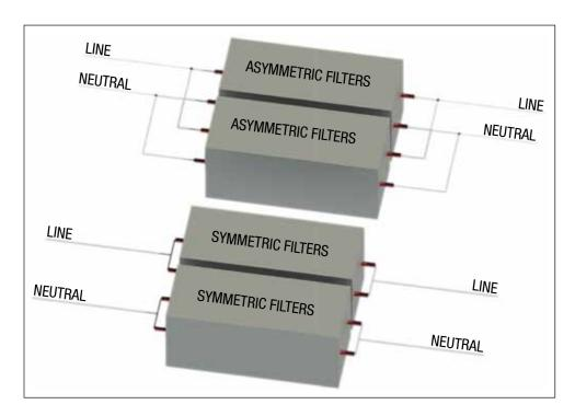
This diagram shows an example of the difference between paralleling asymmetric versus symmetric filters.
